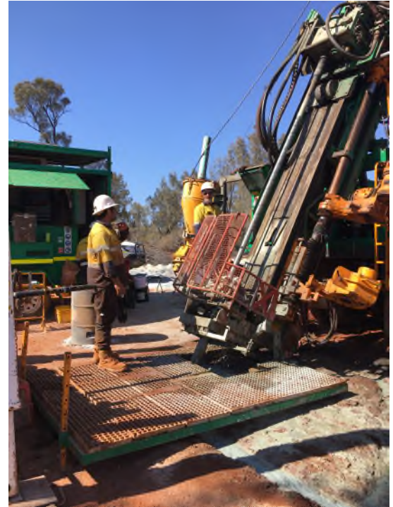
Figure 2, Diamond Drilling at Grey Dam Nickel Project
